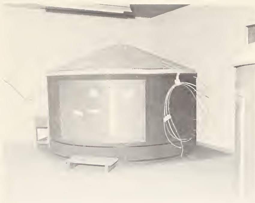
Figure 1.—Experimental storage bin, showing entrance door and plastic roof, simulates 3,250-bushel metal bin.
